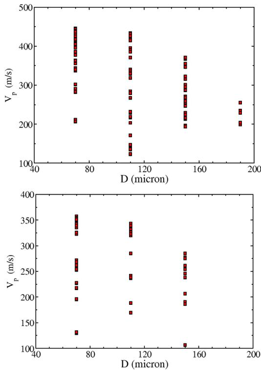
**Figure 7 Particle exit velocities from simulation (Top) Expt. 3 (Bottom) Expt. 4.**
