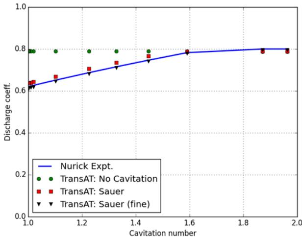
**Figure 4 Predicted discharge coefficient for the sharp edged orifice case of Nurick (Nurick, 1976) and comparison to experimental correlation.**
