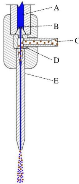
**Figure 1 Sketch of a typical abrasive water jet cutting head.**
