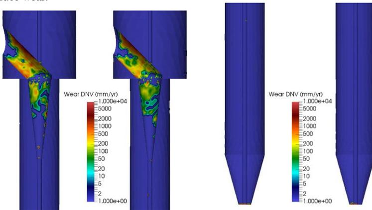
**Figure 8** Wear pattern in mm/yr. estimated using the DNV erosion model (left) Expt. 3, (right) Expt. 4.
