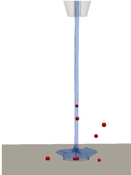
**Figure 6** Snapshots of Expt. 4 simulation in 3D. Near the focusing tube exit.
