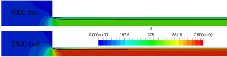
**Figure 3 Hydraulic flip in sharp edged orifice simulated with the cavitation model**
