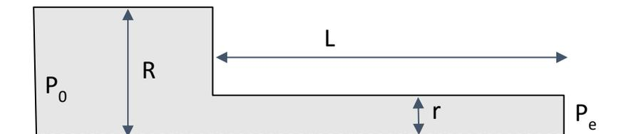
Figure 2 Sketch of the sharp orifice experiment of Nurick (1976).
