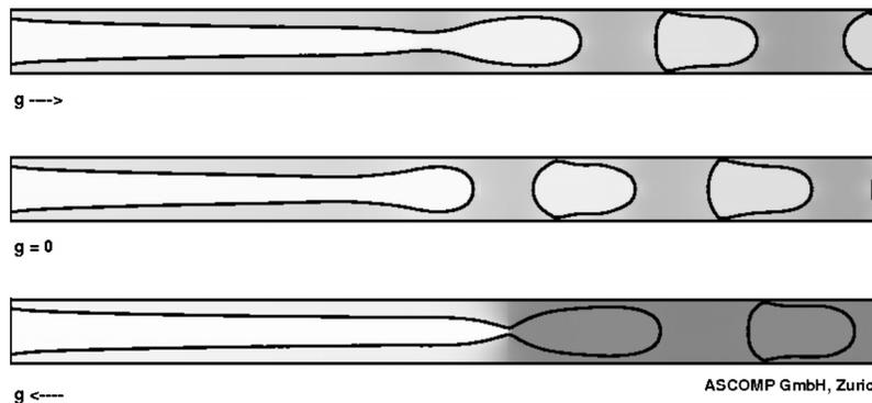
**Fig. 7 Slug breakup under normal- and microgravity conditions**
